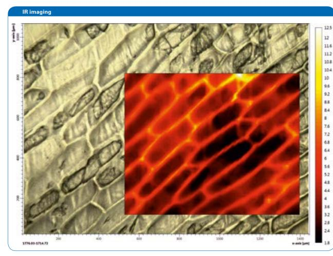
Tissue (onion) measured in transmission with a lateral resolution of 15  $\mu$ m. IR image shows the lipid content of the cells as a 2D false color plot on top of the visual image.
