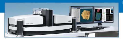
Volume rendering of the cell structure inside wood, 0.5µm isotropic pixel size, 4904x4904x1915 pixels
