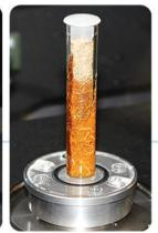
A large number of optional sample mounts are available. Systems can be equipped with tube sample holders for different sample sizes. These allow automated batch scanning, imaging of hydrated samples and samples in liquid. The tube set has four replaceable tube holders with internal diameters of (approx.) 6, 10, 15, and 20 mm.
