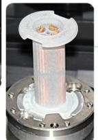
Another optional sample mount is dedicated to scanning several samples simultaneously for comparison. It contains two layers of parallel tube compartments for four samples up to 5mm in diameter. This allows analysis of 8 small samples in a single scan.
