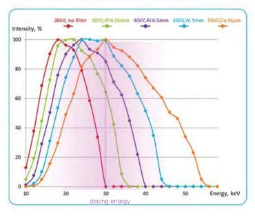
Using the X-ray interferometer for phase-contrast retrieval imposes certain restrictions on the acceptable range of X-ray energies. The system includes an X-ray source with peak energy tunable in the range 20-60 keV and an automatic filter changer with five positions to cut out low X-ray energies. Selecting the proper combination of peak energy in the source and energy filter allows tuning of a narrow band of energies according to the absorption of the object under investigation.
