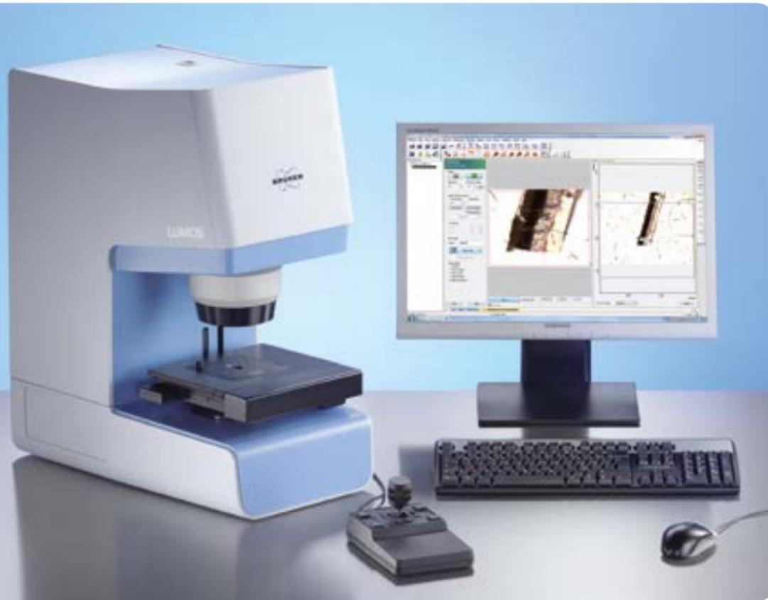
The LUMOS is a very compact stand-alone FTIR microscope. Its dimension (width x height x depth) is just 30 x 64 x 52 cm, requiring less space than conventional FTIR microscopes.
