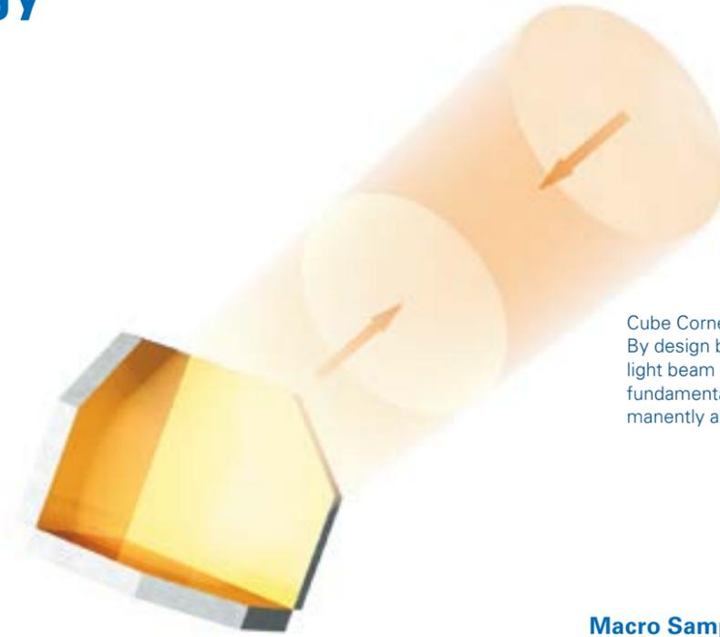
Cube Corner mirrors are immune to mirror tilt. By design both, the incoming and reflected light beam are exactly parallel. This is the fundamental principle of Bruker Optics' permanently aligned RockSolid™ interferometer.
