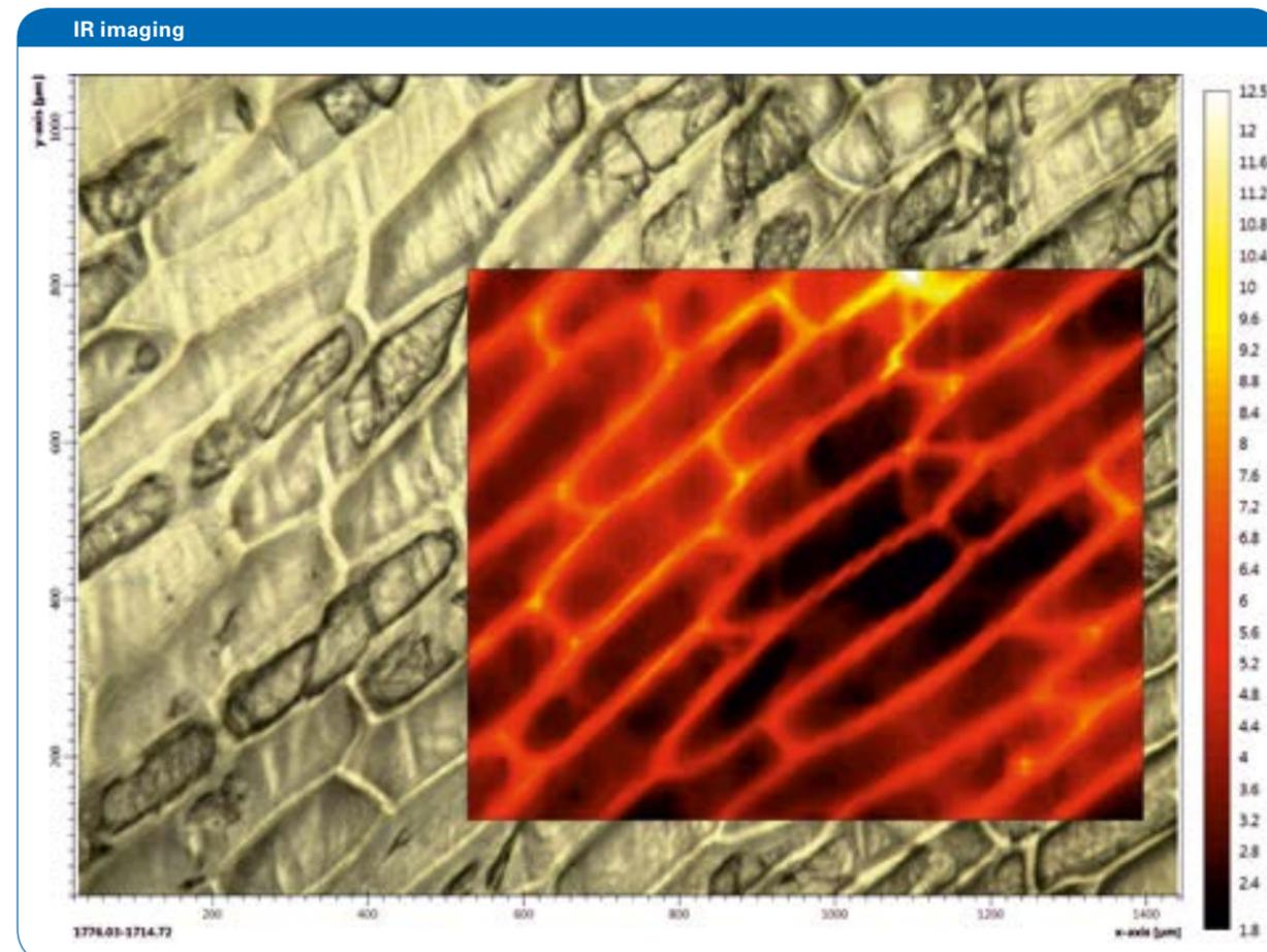
Tissue (onion) measured in transmission with a lateral resolution of 15  $\mu\text{m}$ . IR image shows the lipid content of the cells as a 2D false color plot on top of the visual image.
