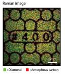
Excitation laser : 532 nm Objective lens : 0.5x Number of pixels : 128 x 128 pixel Measurement time : 0.1 sec / pixel
