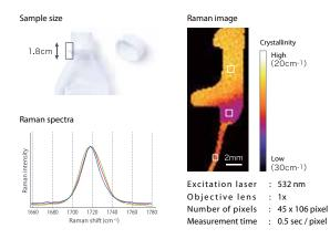
Crystallinity of polyethylene terephthalate corresponds to the width of the Raman peak at 1720cm-1. The Raman image shows the crystallinity of a plastic bottle.
