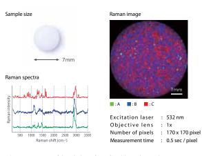
The Raman image of the whole surface of a tablet is shown above. RAMANview visualizes the spatial distributions of multiple components such as medical properties and additives.
