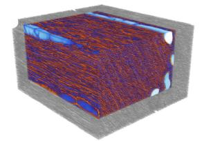
Hartwood, color-coded structure thickness (red) and separation (blue) distribution
