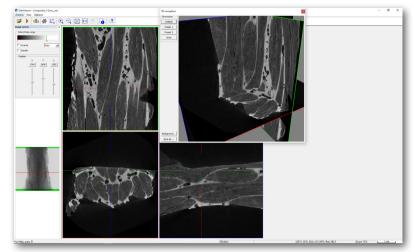
3 orthogonal projections through a CFRP composite
