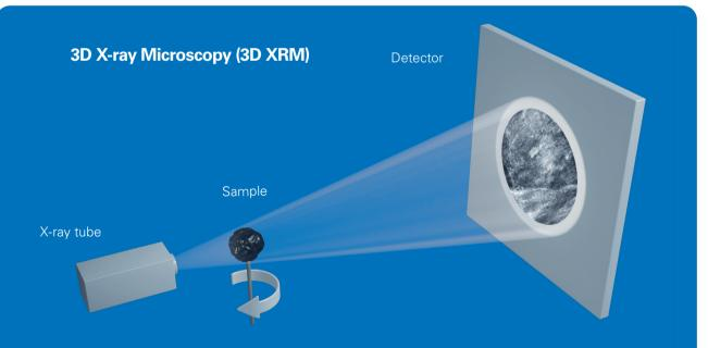
When X-rays pass through an object the intensity is reduced by absorption proportional to the average atomic number along the trajectory.
