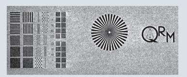
Several factors affect the true 3D spatial resolution: the focal spot size of the X-ray source, the acquisition geometry, the overall system stability, the mechanical accuracy of the rotation axis, as well as the reconstruction algorithms. The 3D spatial resolution is determined with special phantom structures after reconstruction. The SKYSCAN 1272 CMOS easily resolves better than 4  $\mu$ m in both directions.
