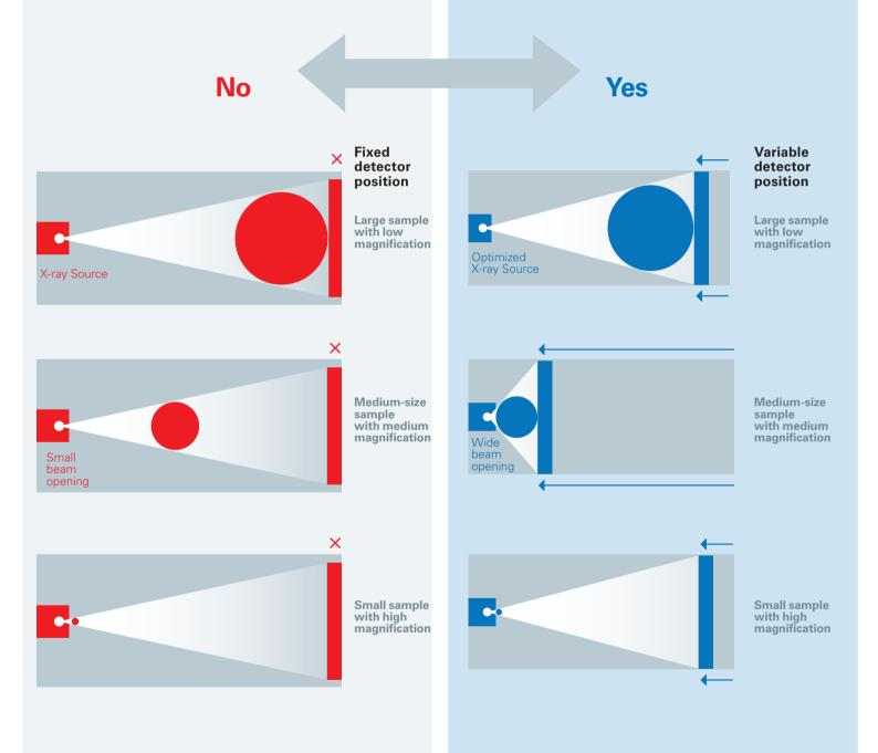
Conventional fixed camera systems are limited to one scanning speed, regardless of the sample size or magnification. Moving both the sample and the sCMOS detector as close as possible to the source increases the measured intensity dramatically. That's why SKYSCAN 1272 CMOS scans faster than conventional systems.
