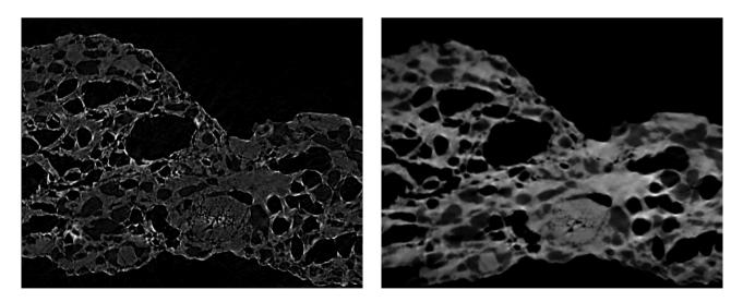
The images show a reconstructed slice through chips. When potato slices are deep fried, oil preferentially fills pores at the surface. With standard absorption contrast (left) it can be challenging to discern between oil-filled and unfilled pores. Applying a phase retrieval algorithm significantly enhances contrast (right).
