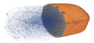
Pharmaceutical tablet, color-coded coating thickness and visualization of pore distribution (blue)
