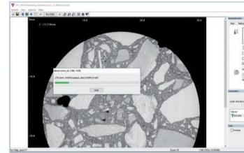
Reconstruction of a concrete core in NRECON
