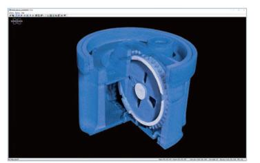
The internal components of an inhaler scanned in just 100 seconds 40 µm pixel size, 100 kV, 1 mm Cu filter, 972 x 972 x 768 px – 38 mm sample diameter
