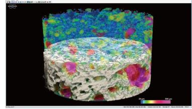
3D reconstruction of the internal microstructure of a carbonate, volume rendering with top half virtually removed overlapped with color map of local pore sizes 20  $\mu$ m voxel size, 80 kV, 1 mm Al filter, 1,944 x 1,944 x 2,925 px – 35 mm sample size
