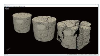
In-situ mechanical testing of a limestone plug under 0, 150 and 500 N of compression 12  $\mu m$  pixel size, 100 kV, 1 mm Cu filter, 1,944 x 1,944 x 1,536 px – 10 mm sample size
