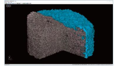
Volume render of salt crust on a Bentheim sandstone. 5  $\mu m$  voxel size, 80 kV, 1 mm Al filter, 1,944 x 1,944 x 1,536 px – 6 mm sample diameter
