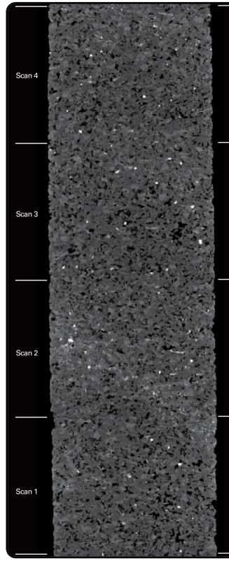
Automated stitching of multiple circular scans of a sandstone microplug 5  $\mu$ m voxel size, 80 kV, 1 mm Al filter, 1,944 x 1,944 x 6,000 px – 5 mm sample diameter
