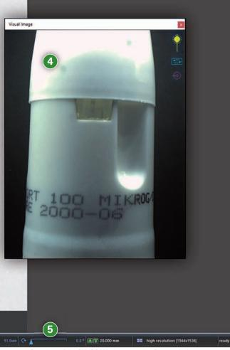
Overview of the SKYSCAN 1275 control software window Inhaler, 40  $\mu m$  voxel size, 100 kV, 1 mm Cu filter, 972 x 768 px
