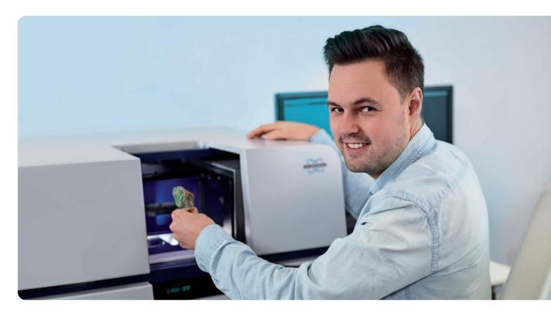
The SKYSCAN 1275 is an unparalleled desktop 3D X-ray microscope based on micro computed tomography (Micro-CT). This non-destructive imaging technology, pioneered by Bruker, uniquely provides 3D insights into samples of any material, any shape, and any size with little to no sample preparation. SKYSCAN 1275 makes this attractive technology available to everyone. This desktop instrument fits in every lab and excels in easy-of-use thanks to the high level of automation.
