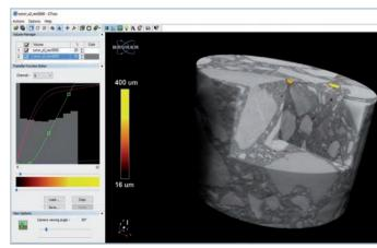
Volume rendered concrete sample showing color-coded pore size distribution in CTVOX
