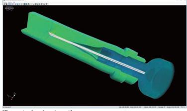
3D reconstruction of a syringe with a cap 8 µm voxel size, 70 kV, 1 mm Al filter, 1,944 x 1,944 x 3,980 pixels – 6 mm sample size
