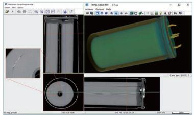
Orthogonal slices and volume render of a large capacitor. 25 μm voxel size, 100 kV, 1 mm Cu filter, 1,944 x 1,944 x 6,000 px – 40 mm sample diameter
