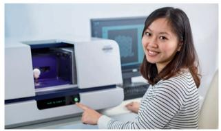
SKYSCAN 1275 high-speed X-ray microscope with Push-Button-CT
