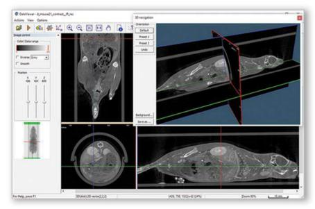
DataViewer shows reconstructed results as a slice-by-slice movie or as three orthogonal sections, intersecting at any selected point in the reconstructed space. One can rotate / reslice the reconstructed volume in any direction. Additional features include the 4<sup>th</sup> dimension for time-resolved cardiac and respiratory tomography, variable smoothing options, measuring distances in 3D with saving a table of results, and measuring intensity profiles.
